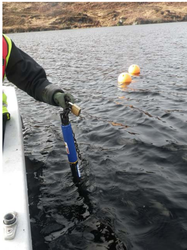
Figure 8: The sonde being installed at 8 m depth in Loch Grannoch
