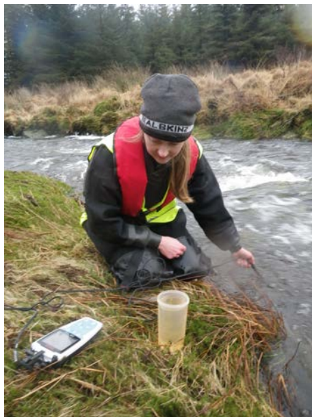
Figure 5: Taking a water sample and measuring the pH of the Cuttiemore Burn
