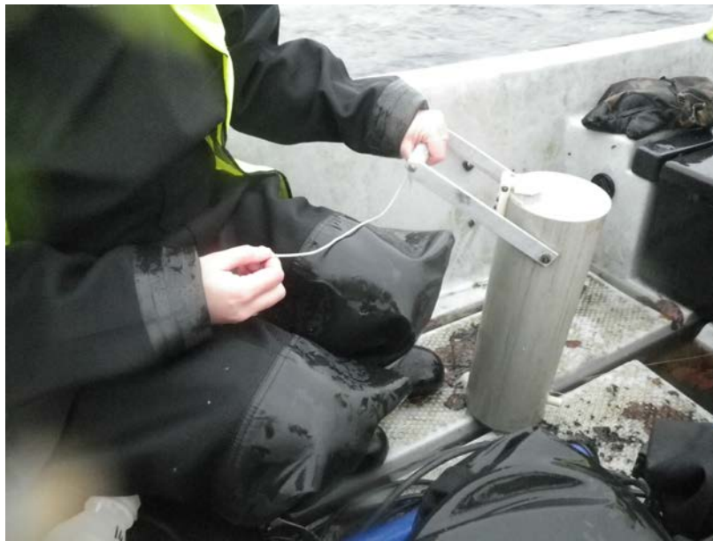
Figure 6: The depth water sampler used to collect water from c.20 m deep for analysis
